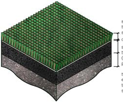
synthetic carpet typically 8-24mm sand fill carpet backing shockpad typically 8-25mm (In-situ, prepared or prefabricated)
